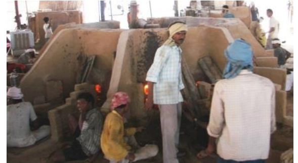
Traditional reheating furnace
