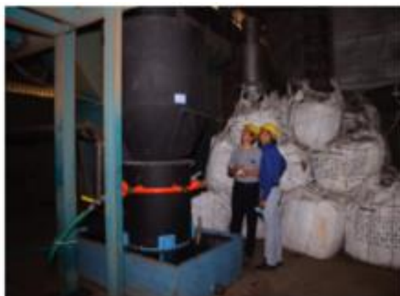
Biomass Gasifier for Sand Drying at Belgaum Foundry Cluster
