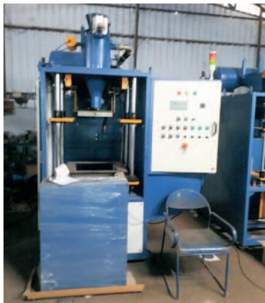
Core Modification Process through Cold box core shooter
