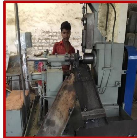
SPM - turning installed at Mehram Industries
