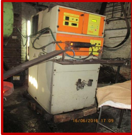
Induction heater installed at C-Forge (India)
