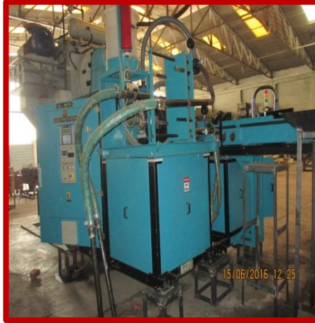
Induction heater installed at Global exports
