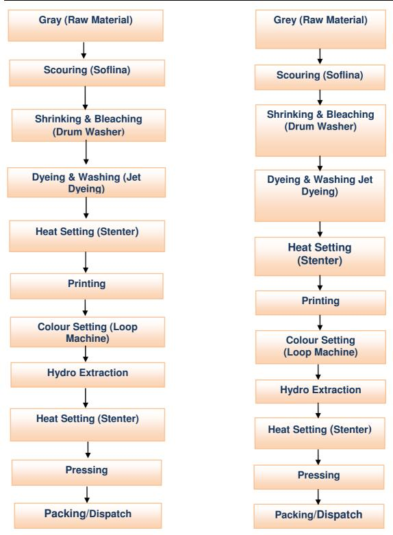
Figure 1.1 Process Flowchart of Surat Textile Cluster
