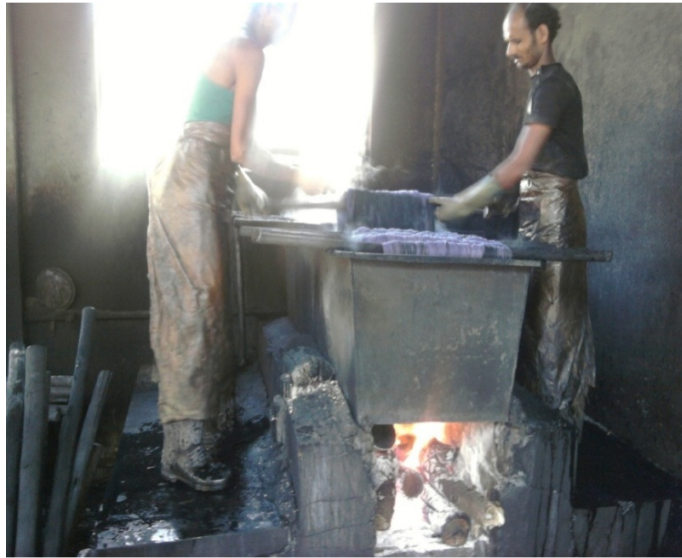
Figure 1.2 Conventional chulhas operation at textile industry
