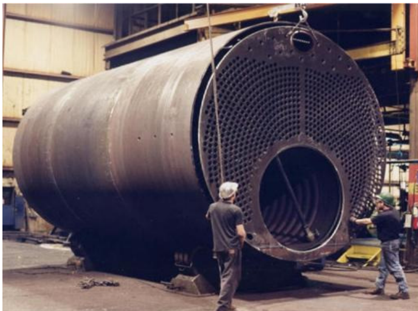
Fig. 1.9 – Typical Arrangement of tubes in Boiler
