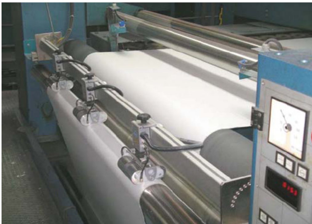
Fig. 2.2 Residual moisture measurement and control system installed in a stenter
