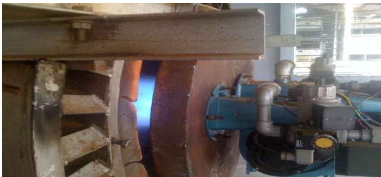
Figure 2: Side View of the Energy Efficient Burner
