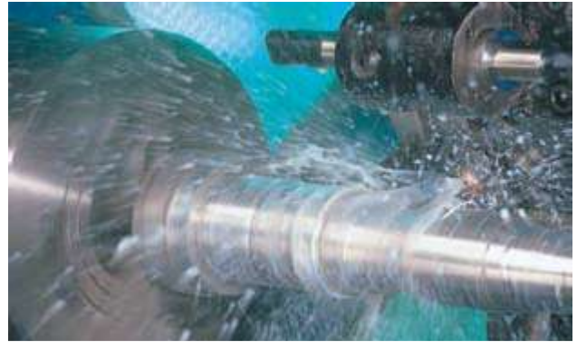
Coolant is supplied through the turret and ejected through the tool holder to allow the coolant to reach the cutting point more effectively.
