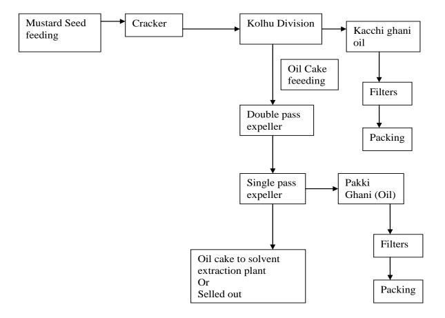
Figure 1.1: General process flowchart of a typical Oil mill
