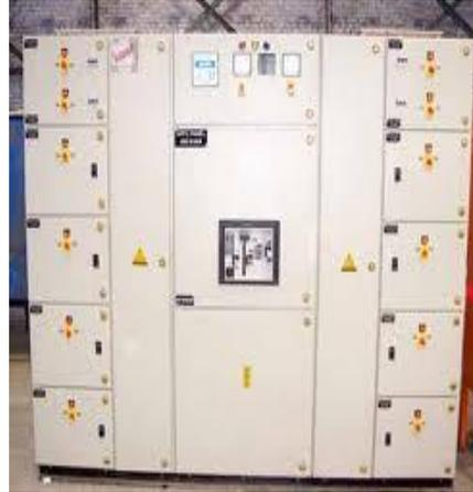
An automatic power factor correction unit is used to improve power factor. A power factor correction unit usually consists of a number of capacitors that are switched by means of contactors. These contactors are controlled by a regulator that measures power factor in an electrical network. To be able to measure power factor, the regulator uses a current transformer to measure the current in one phase.
