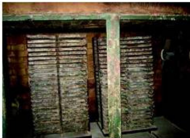
Figure1.2 Tray dryers operations at a chemical industry
