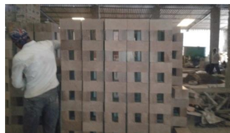
Natural drying in downdraft kilns
