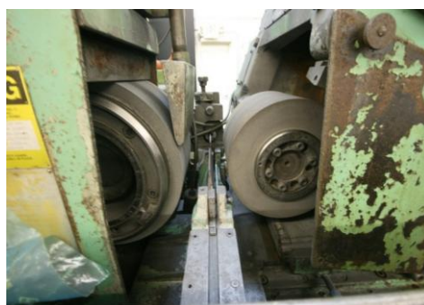
Centre-less grinding machine for race O.D grinding
