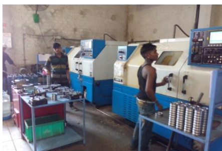
Race finish turning on CNC machine
