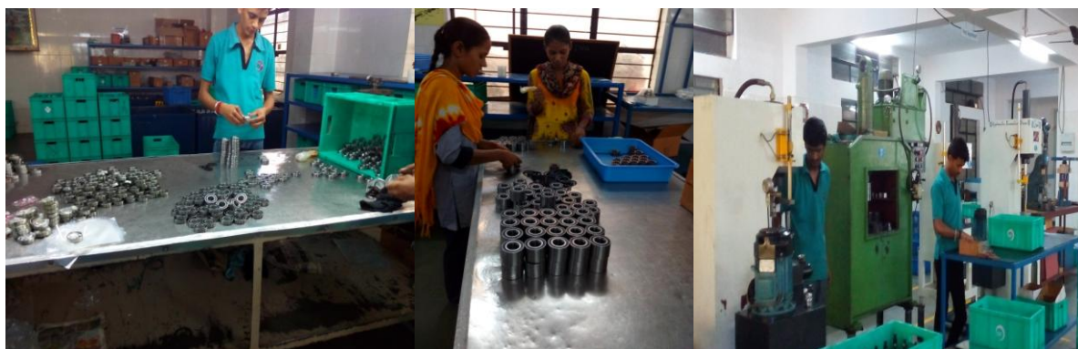
Bearings manual assembly line
