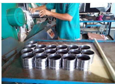
Centre-less grinding machine for race O.D grinding
