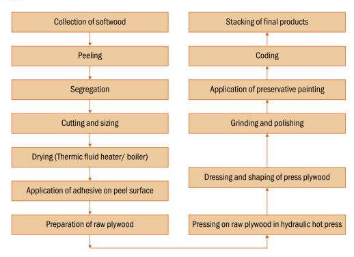
Process flow diagram of plywood manufacturing
