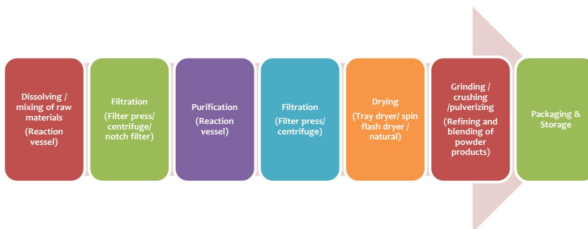
Figure4.1b: Process flow in typical dyes and pigment manufacturing units
