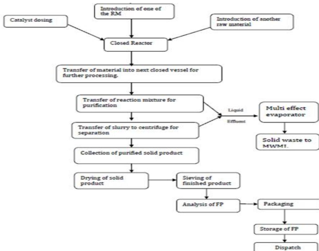
Figure4.2: Prodction process of Anti-oxidant
