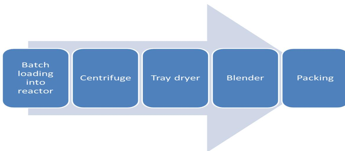
Figure 4.3: Production process of Bulk drugs
