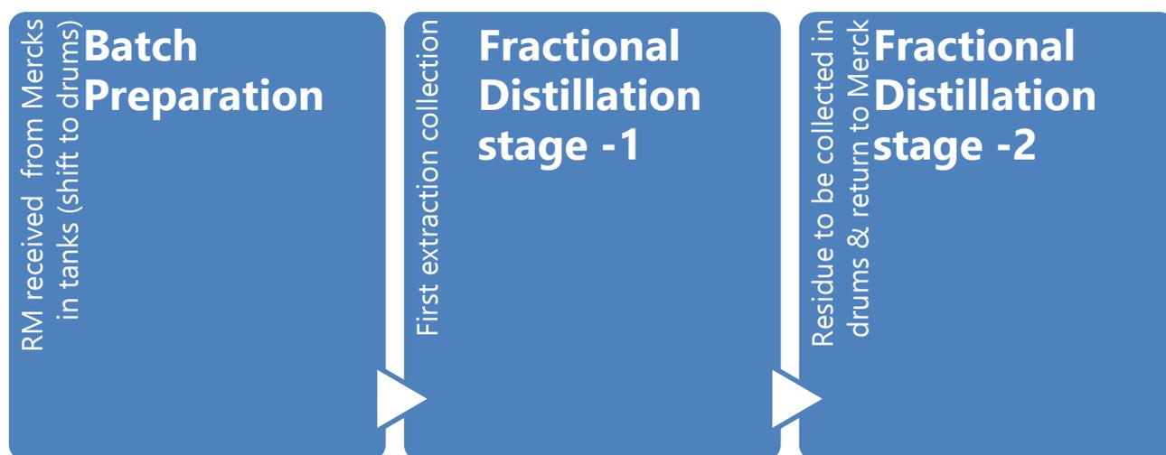
Figure 4.1: Production process of Solvent Distillation
