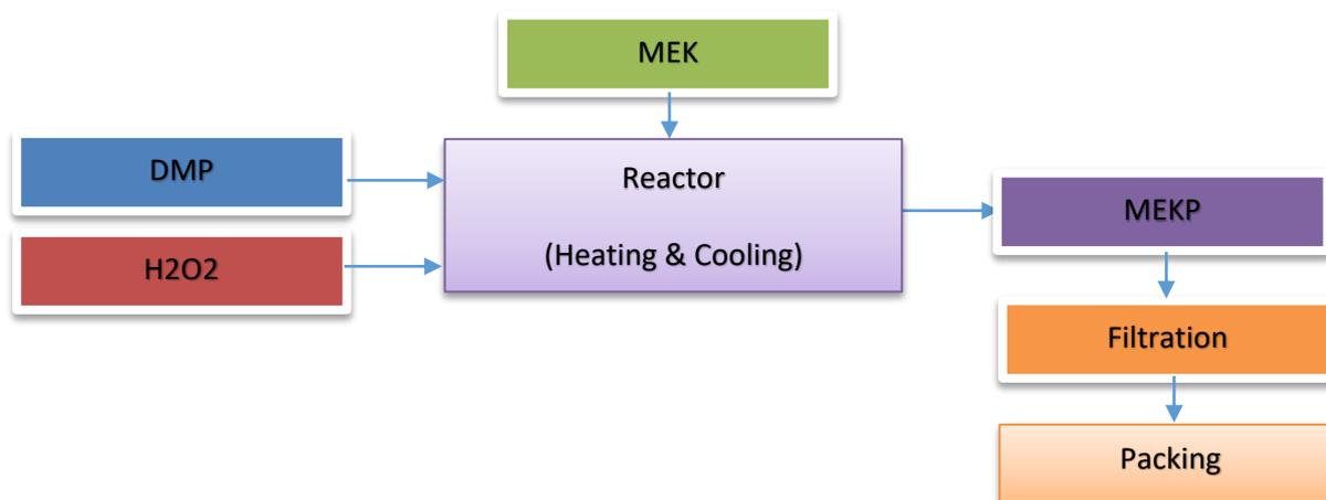
Figure 4.4: Production process of Resin
