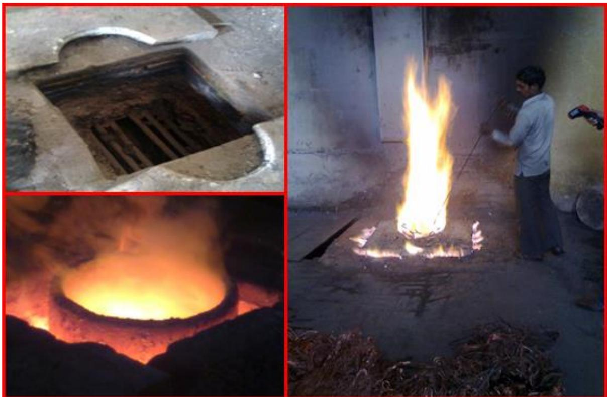
**Figure 7: The pit furnace design and the photographs taken during normal operational**
