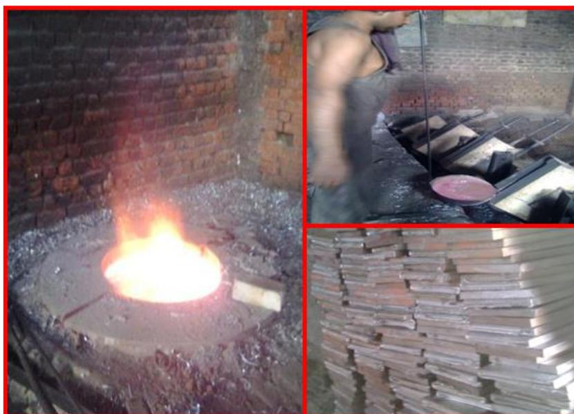
**Figure 9: The pit furnace design and the photographs taken during normal operational**
