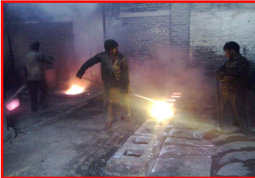
**Figure 8: Casting process photographs taken during normal operational OIL FIRED PIT MELTING – ALUMINIUM MELTING UNITS**
