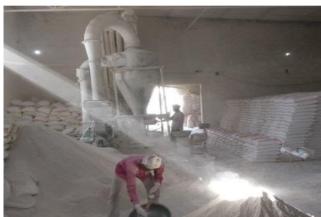
Mixing and pulverizing of POP
