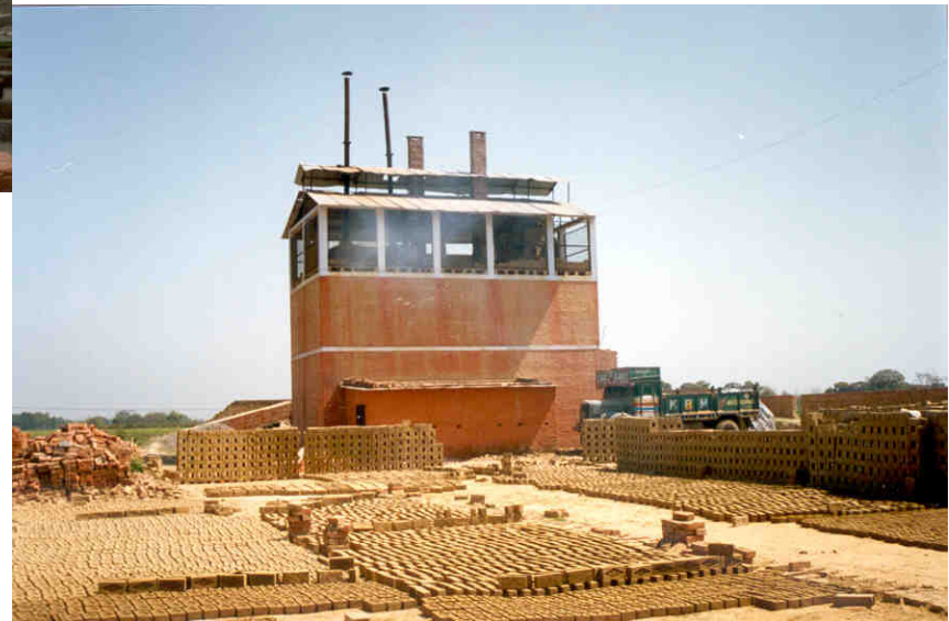
Vertical Shaft Brick Kiln (VSBK)
