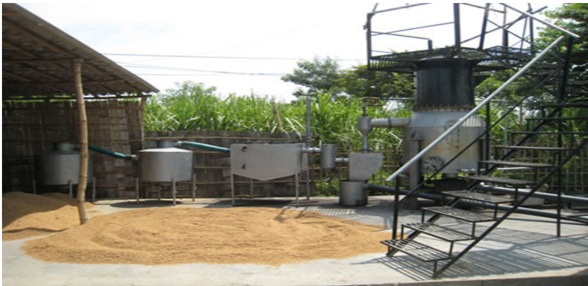
Figure 2.1: Bio Mass gasifier
