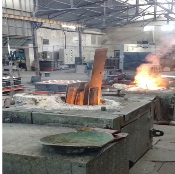
Energy inefficient operating practice: large sized raw materials charged into induction furnaces
