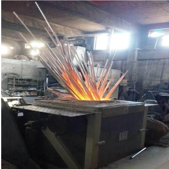
Energy inefficient operating practice: large sized raw materials charged into induction furnaces
