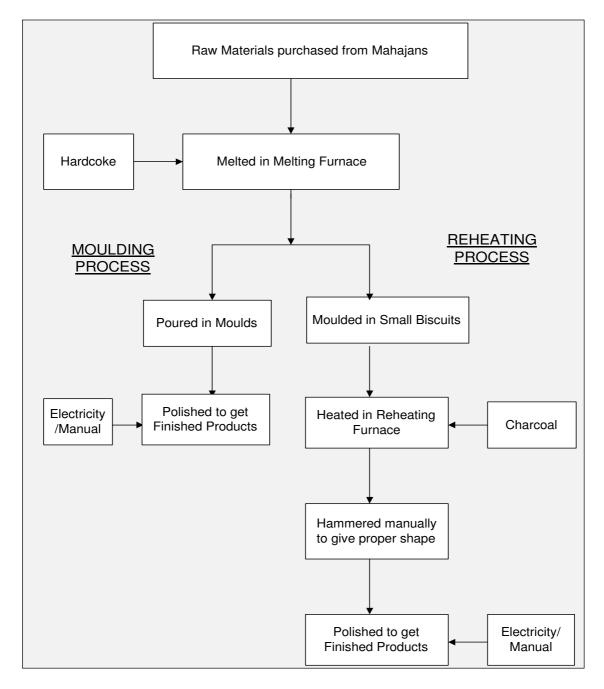
Figure 1.3 Process Flow Diagram of manufacturing of Brass Unit
