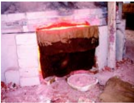
(ix) Soaked gunny bag placed over gap in furnace wall
