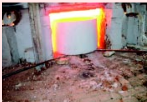
(iv) Introducing trial pot into pot furnace
