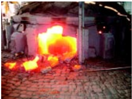
(iii) Wall dismantled, showing failed pot inside furnace
