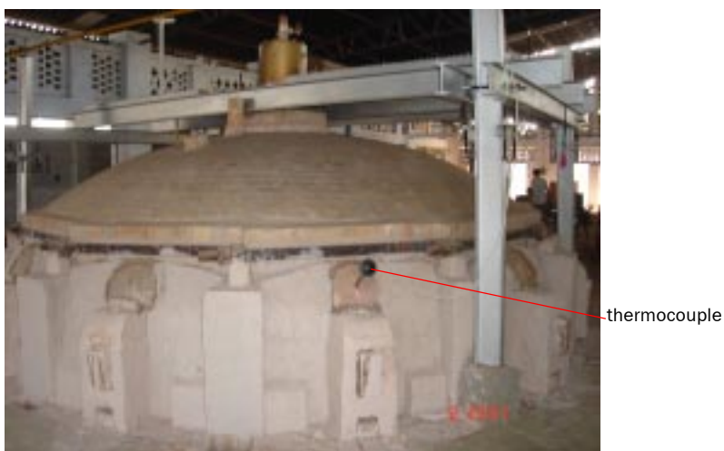
Figure A2-1 Measuring furnace temperature
