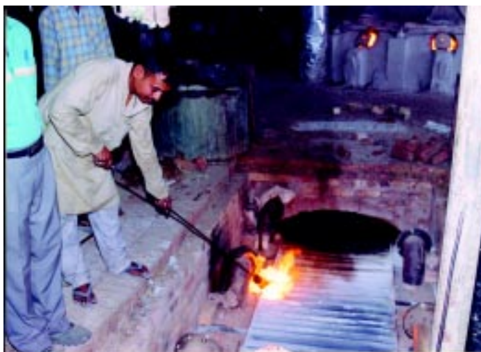
Figure 50 Testing for leakages with a palita
