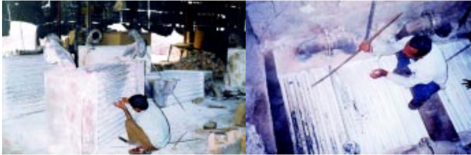
Figure 34 Cleaning the recuperator modules
