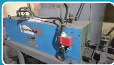
FO-fired bath replaced with electric induction heater at a wire-drawing unit in Ranchi
