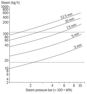
Figure 2 Steam losses from various leakage sizes and pressure
