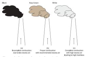
Figure 1 Colour of smoke from boiler chimney
