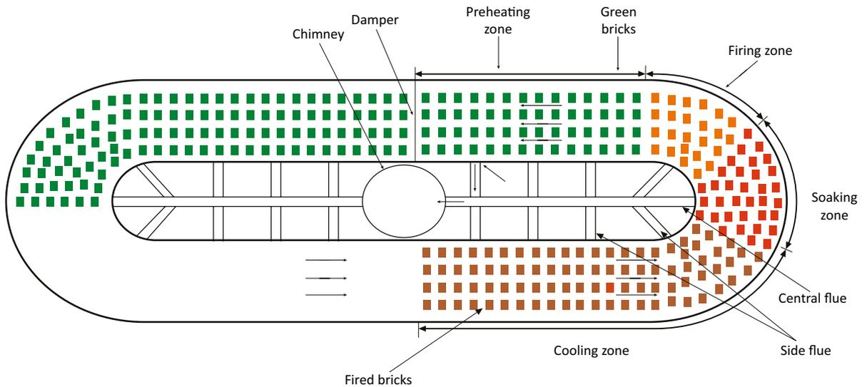
*Schematic diagram of a BTK*
