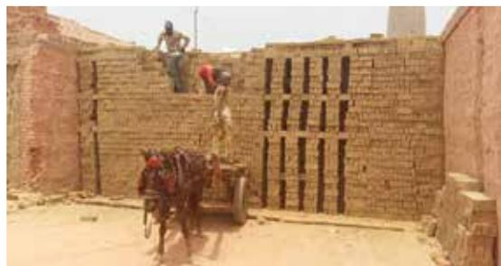
*Brick stacking in zig-zag firing process*
