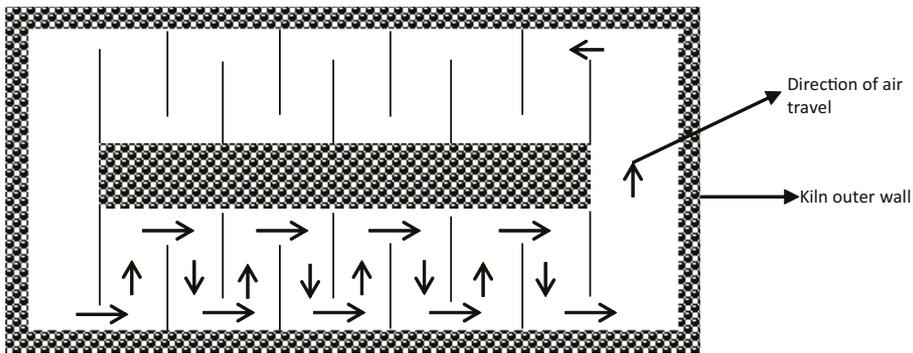
*Direction of air flow in single zig-zag firing process*
