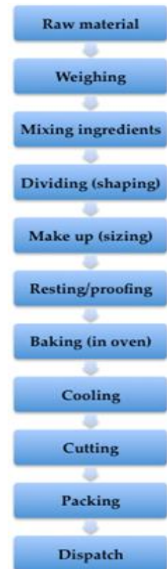
Production process of a bakery unit
